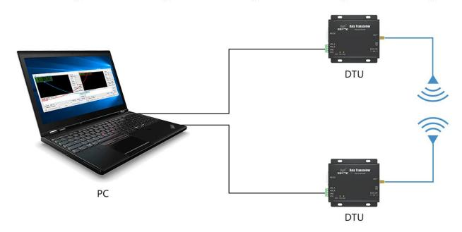
3、 Firing up two XCOMs, choosing Baud rate 9600bps, 8N1, the setting which serial port transmission can be achieved.
