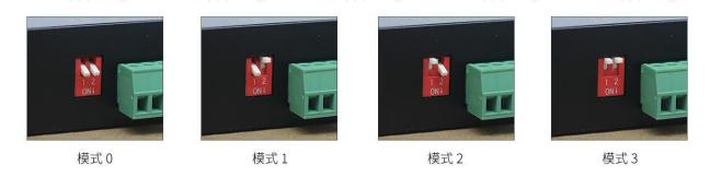
★ Note: no need to care about the wake-up mode (mode 1) and power saving mode (mode 2) if it doesn't request low power consumption.
