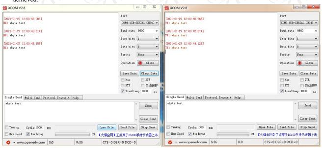
4、 User needs to open the mode switch first before link DTU with computer if the user want to modify parameters. Firing up <u>E32-DTU 数传电合配置软件(E32-DTU</u> parameter configuration application) to modify related parameters. The mode switch must be reopened to achieve transmission after the configuration.
